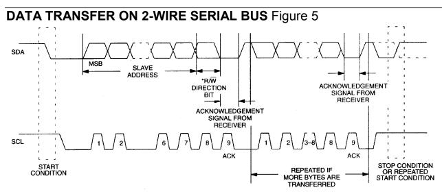
Depending upon the state of the  $R/\overline{W}$  bit, two types of data transfer are possible:
