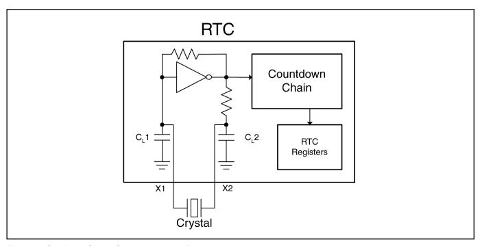
Figure 3. Oscillator Circuit Showing Internal Bias Network
