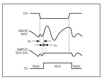
Figure 10. T/H Aperture Timing
