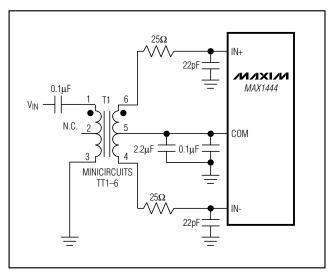
Figure 8. Using a Transformer for AC Coupling
