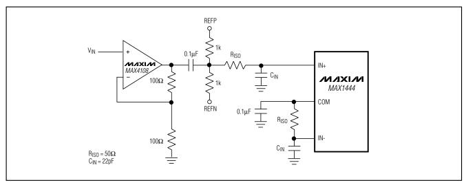
Figure 9. Single-Ended AC-Coupled Input
