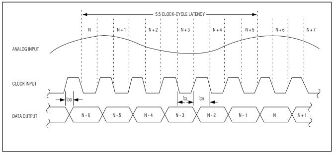
Figure 6. System and Output Timing Diagram
