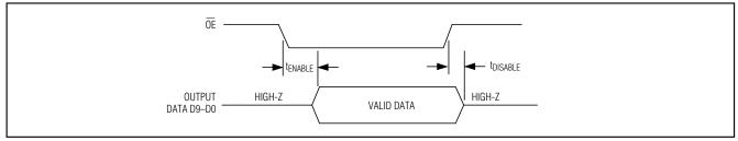
Figure 5. Output Enable Timing
