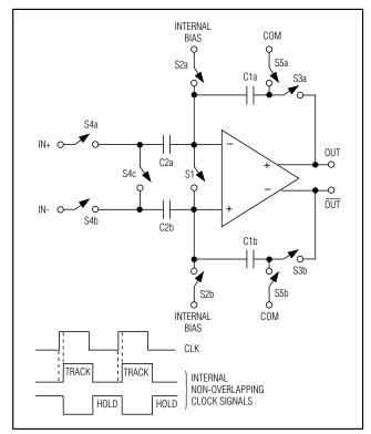
Figure 2. Internal T/H Circuit
