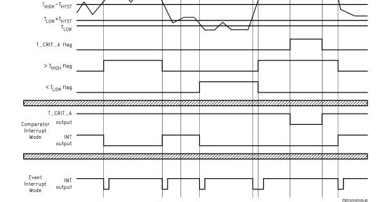
Note: Event Interrupt mode is drawn as if the user is reading the part. If the user doesn't read, the outputs would go low and stay that way until the LM76 is read. FIGURE 3. Temperature Response Diagram
