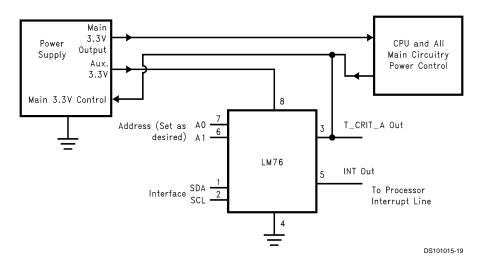
FIGURE 9. ACPI Compatible Terminal Alarm Shutdown. By powering the LM76 from auxilary output of the power supply, a non-functioning overheated computer can be powered down to preserve as much of the system as possible.
