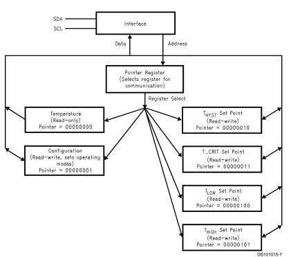
There are four data registers in the LM76, selected by the Pointer register. At power-up the Pointer is set to "00"; the location for the Temperature Register. The Pointer register latches the last location it was set to. In Interrupt Mode, a read from the LM76 resets the INT output. Placing the device in Shutdown mode resets the INT and T\_CRIT\_A outputs. All registers are read and write, except the Temperature register which is read only.
